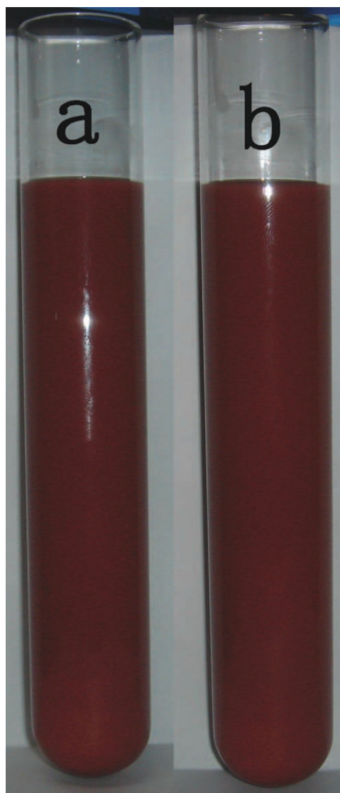
Figure 7. The photos of the dispersions (a) before and (b) after 2 months of storage. [Color figure can be viewed in the online issue, which is available at wileyonlinelibrary.com .]
